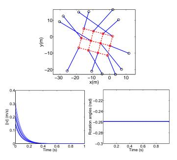
Fig. 4. Simulation results using the proposed control scheme with time delays  $\tau_{ki} = \bar{\tau} = 500ms$  and no delay mismatches  $(\hat{\tau}_{ki} = \tau_{ki})$ . Upper figure: trajectories followed by each agent converging to the desired geometric configuration. Lower left-side: Norm velocities of each agent, Lower right-side: Estimation of the rotation angle  $\hat{\alpha}_i = \hat{\alpha}_0 = -0.2591$ , computed by each agent.
