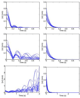
Fig. 7. Norm velocities corresponding to each agent under time delays: left column, no delay compensation; right column, delay compensation with delay mismatch of 15ms. Top:  $\bar{\tau} = 100ms$ , Middle:  $\bar{\tau} = 200ms$ , Bottom:  $\bar{\tau} = 500ms$ .
