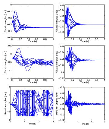
Fig. 6. Estimation of the rotation angle by each agent under time delays: left column, no delay compensation; right column, delay compensation with delay mismatch of 15ms. Top:  $\bar{\tau} = 100ms$ , Middle:  $\bar{\tau} = 200ms$ , Bottom:  $\bar{\tau} = 500ms$ .
