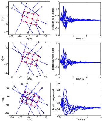
Fig. 9. Simulation results with upper bounde delay  $\bar{\tau} = 500ms$ and bigger delay mismatches: left column, trajectories followed by each agent converging to the desired geometric configuration; right column, estimation of the rotation angle by each agent. Top:  $e_{\tau} = 75ms$ , Middle:  $e_{\tau} = 125ms$ , Bottom:  $e_{\tau} = 250ms$ .
